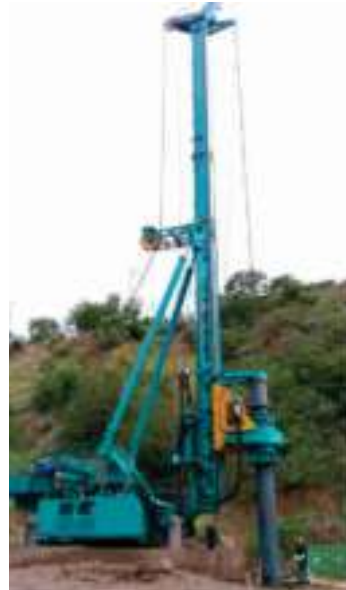
SWDM600W Yunnan high-speed cross Red River grand bridge construction, bearing a complex geological condition with backfill, boulders, gravel layers and other strata. The construction adopted the technology of vibrating hammer retaining cylinder and mud protection wall. The pile diameter is 2.5m, the drilling depth is 72m, and the drilling time is 39 hours for each pile
