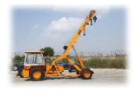
2 LIFTING HEIGHT Higher lifting height of 9 mtrs.
