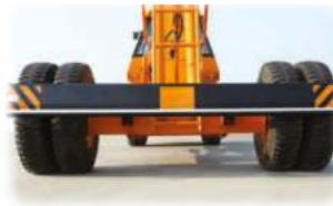
2 GROUND CLEARANCE High ground clearance of 400mm for easier rough terrain operation.
