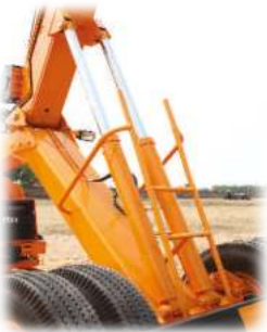
ACE 18XW 4-Part Boom (20 Mtrs. Height) Max. Capacity Manual Extension : 2 Tonnes
