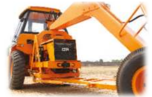
3 STEERING CYLINDERS 880 mm stroke cylinders ensure proper steering even in loose, sandy & rocky terrains.
