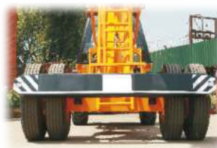
2 GROUND CLEARANCE High ground clearance of 400mm for easier rough terrain operation.
