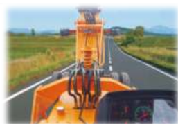
5 INCREASED VISIBILITY Bigger size front windscreen and re-routing of hoses provide much better front visibility.
