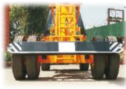
6 GROUND CLEARANCE High ground clearance of 400mm for easier rough terrain operation.
