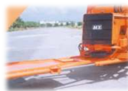
7 STEERING CYLINDERS 700 mm stroke cylinders ensure proper steering even in loose, sandy & rocky terrains.
