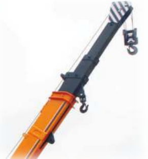
8 SLOTTED BOOM For easier load positioning
